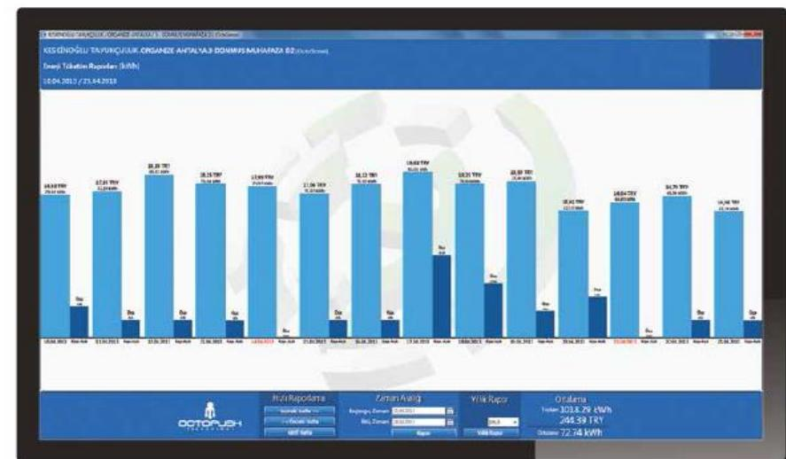
By entering a certain time interval, you can monitor the cold room's energy consumption on kWh and price basis as well as the daily door-open times.
